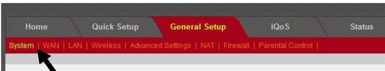
You can configure your time zone, password, and remote management settings here. After you have completed the configurations, click “Apply” to save the changes.
