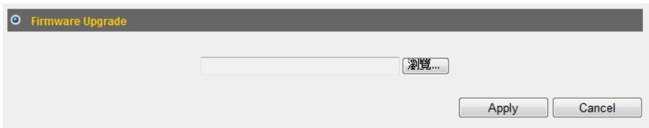
2. Click “Browse...” to find the firmware file saved on your computer, then click “Apply” to start firmware upload. The broadband router will restart after the file is uploaded. All your current settings will be lost after the firmware is upgraded.
